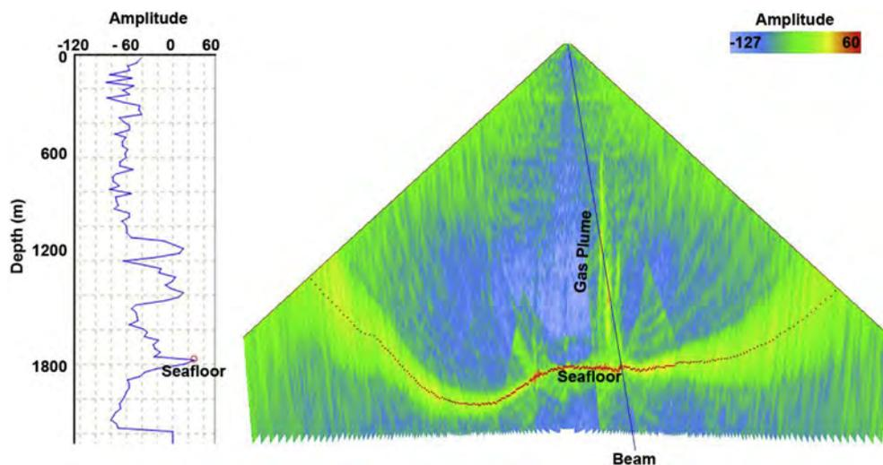
**Figure 5.** Site 1 beam fan with time series amplitude versus range (m) for a nearly vertical beam ( $\sim 20^\circ$  off nadir). Note that the flare is characterized by positive amplitudes higher than background water column values. The location of Site 1 is given in Figures 1 and 2, for color map see Figure 4. (For interpretation of the references to colour in this figure legend, the reader is referred to the web version of this article.)
