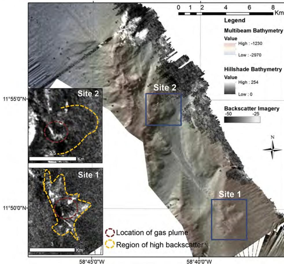
**Figure 3.** Base map: Sites 1 and 2 imaged by draping transparent multibeam bathymetry and hillshade layers over backscatter imagery. Illumination is cast from 315° at an altitude of 30°. Insets: regions of relatively high backscatter that cover the seafloor at sites 1 and 2.
