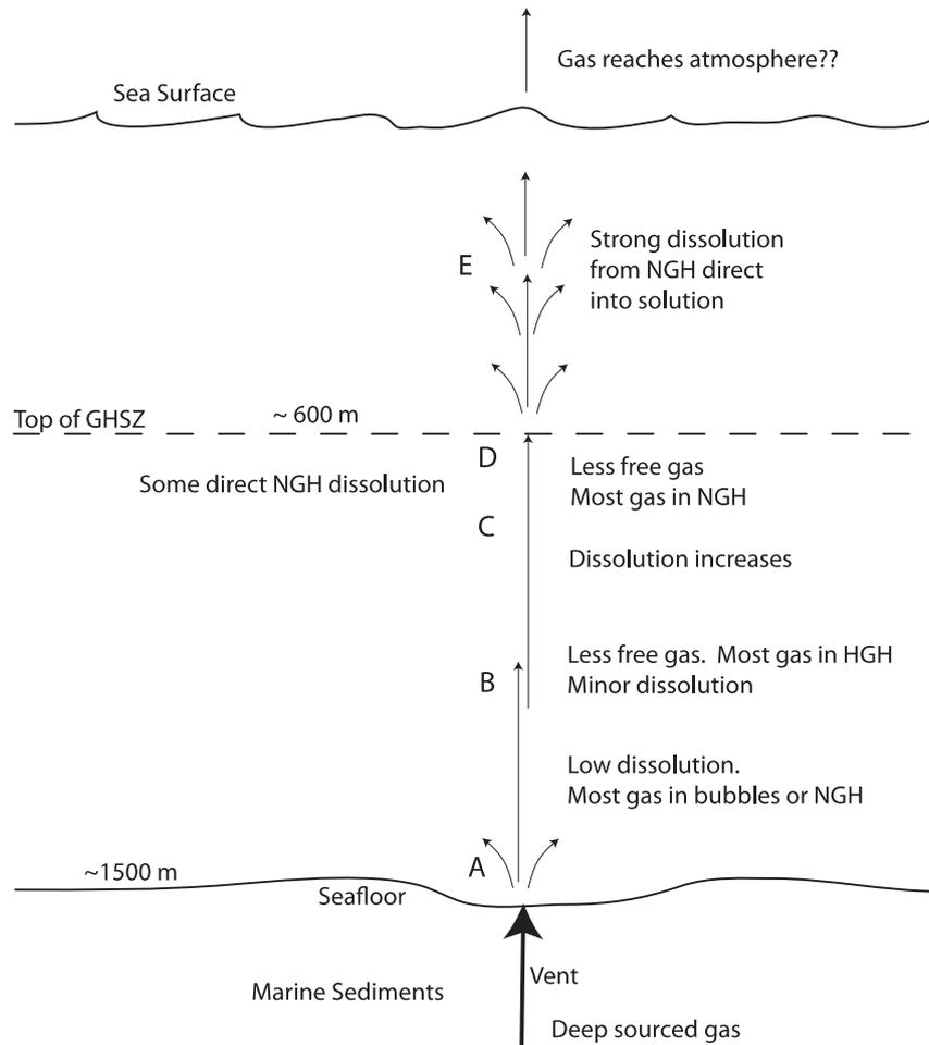
**Figure 8.** Schematic representation of ascending gas/NGH from vent toward sea surface.
