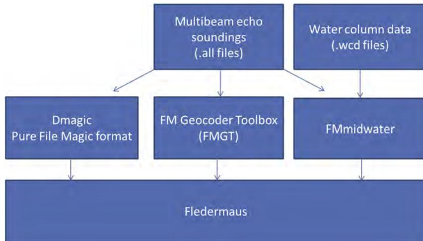
**Figure 2.** QPS multibeam processing workflow including the modules used. The Dmagic module processes multibeam data into multi-resolution bathymetric surfaces, FM Geocoder Toolbox creates qualitative and quantitative acoustic backscatter mosaics, FMmidwater allows the visualization and analysis of water column data, and the Fledermaus module integrates data from all the modules and allows visualization.
