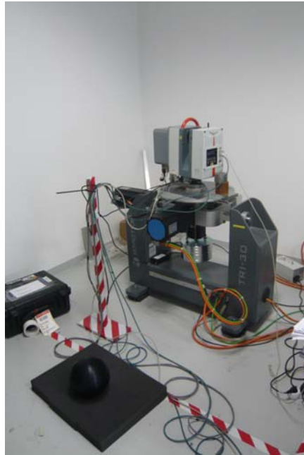
Figure 2: Experimental set-up for latency calibration: The Leica HDS6200 and the IxSea Octan4 are mounted on a IXMotion TRI30 motion simulator, scanning a sphere of precision.
