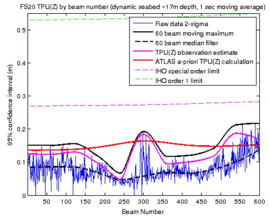
Figure 7: Maximum-median estimated vertical TPU using data contributing to the uncertainty surface in figure 6
