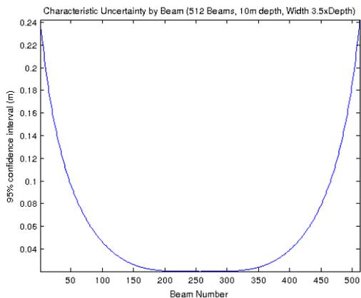
Figure 1: Characteristic distribution of vertical TPU for a typical beam-forming sonar, 10m depth 350% coverage.
