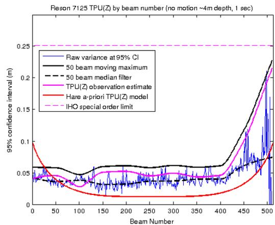
Figure 8: Reson 7125 calculated (red) and maximum-median estimated (magenta) TPU. Stationary vessel.
