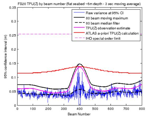
Figure 4: ATLAS FS20 a-priori calculated (red) and maximum-median estimated (magenta) uncertainty over a consistent sea-floor; 3 second along-track average, 80 beam across track filtered.
