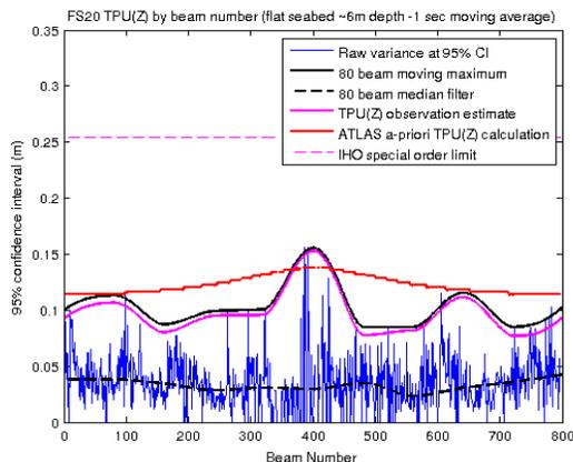
Figure 3: ATLAS FS20 maximum-median estimated (magenta) and a-priori calculated (red) uncertainty. Consistent seabed in optimal conditions. 1 second along-track averaging, 80 beam across track filtering.
