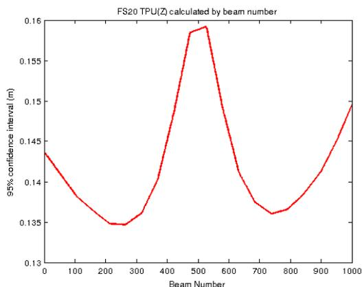
Figure 2: ATLAS Fansweep 20 a-priori vertical TPU distribution. 14m depth, 1000 beams, 1000% depth coverage.
