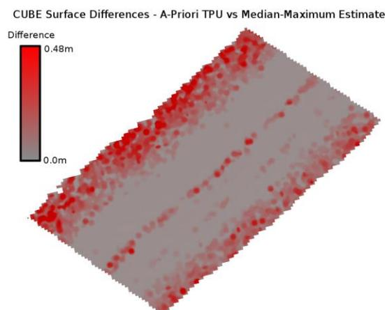
Figure 10: CUBE Surface Differences: a-priori - maximum-median derived vertical TPU
